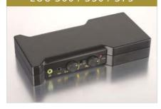
**Dual Channel EOU 300** supports monitoring with two sensors simultaneously. It features two pairs of ST fiber optic connectors; two 3.5 mm stereo sockets (one for analog output, another for headphones); dual volume control knobs; green/red LED voltage indicator. **EOU 350** adds a DSP for up to 22 dB of real-time ambient noise removal (three levels: low, mid, high). **EOU 375** includes DSP as well as 16-bit uncompressed SD Flash memory card recorder.
