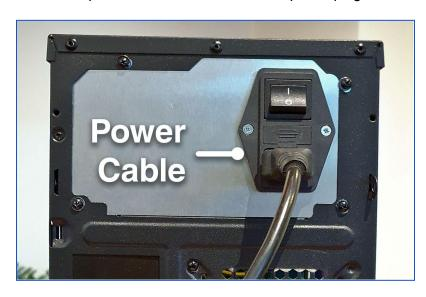
Then connect the power plug at the other end of the cable to a standard electric power supply receptacle. **Do not power on the EOU yet.**
