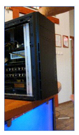
Apply slight finger pressure at the bottom of the panel to release it from the EOU.
